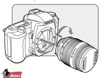
· After attaching the lens, try and turn the lens counterclockwise to make sure it is locked in place.
